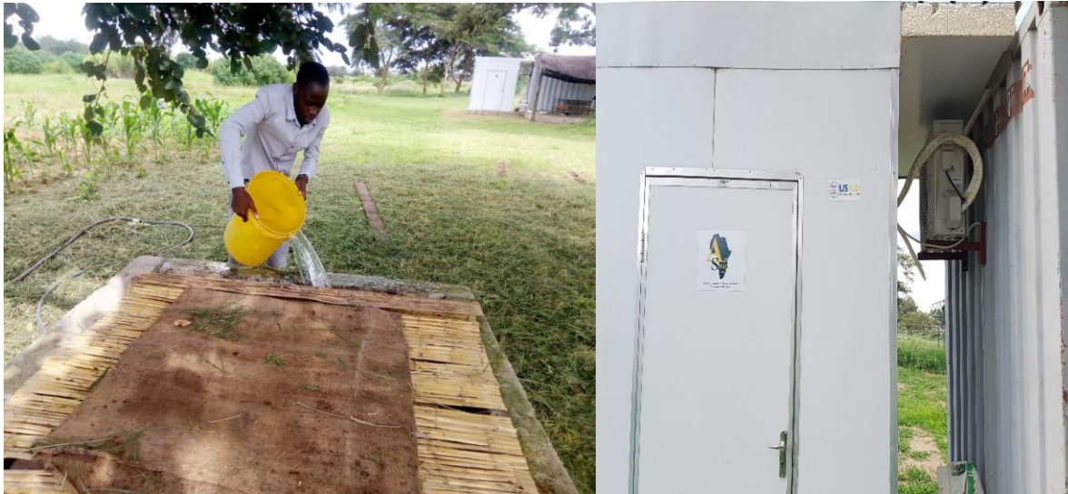
Figure 6. Small sized Zero Energy Cool Chamber (ZEEC) (left) and a COOLBot™ (right) for demonstration and research purposes at the School of Agricultural Sciences of the University of Zambia.
